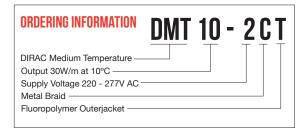
DMT is an industrial grade, self-limiting heating cable that can be used for freeze protection or temperature maintenance to 135°C.
